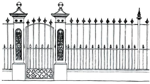
Height @ 1615mm Width of cap @ 400mm Width of Post @ 245mm Width of Base @ 345mm Weight – 41.00kg
